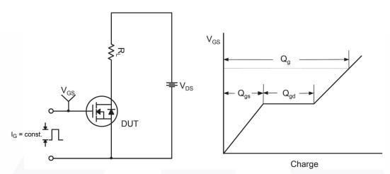
Figure 12. Gate Charge Test Circuit & Waveform
