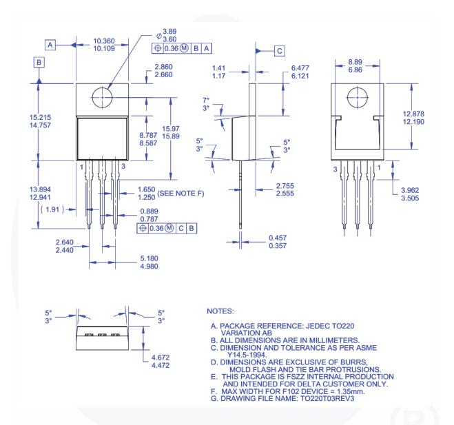
Figure 16. TO-220, Molded, 3-Lead, Jedec Variation AB (Delta)
